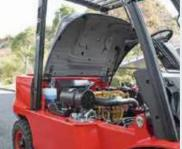
The enlarged opening angle on hood and increase of left and right hood side plates can provide you with convenient and rapid maintenance mode.
