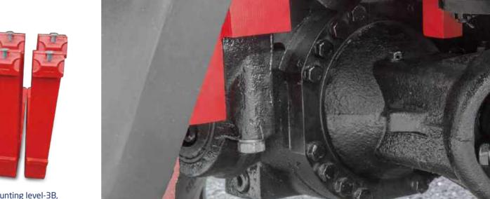
Oscillating steer axle allows either wheel to step over obstacles keeping the truck and load level.
