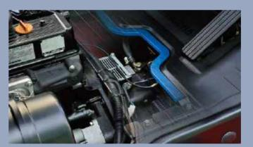
In addition to rubber damper between frames and steering as compound engine damper and full floating power train achieved flexible connection between frames and driving system, as a result, traveling vibrations and vibrations from the driving system are significantly reduced.
