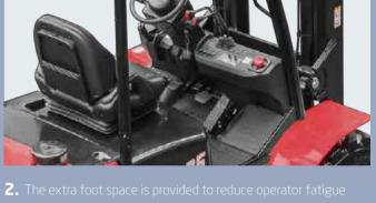
2. The extra foot space is provided to reduce operator fatigue significantly, non-slip step makes getting in and out easy an safe. The new designed steering wheel new brake system and the easy-to-operate levers provide total handling operation.
