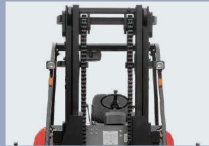
The new wide-view mast enables an excellent view and faster and safer operations
