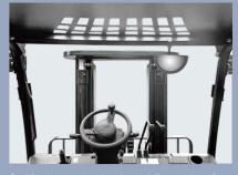
A wide-view mast system is used, the opening of the mast is widened, and the dashboard in the cab is lowered, so that the front view of the driver is broadened significantly
