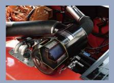
The novel high-flow air filter with a safety filter cartridge to enable cleaner air intake and higher power of the engine
